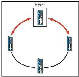
For **Turbo Ring V2**, the backup segment is the segment connected to the 2nd redundant port on the master.
